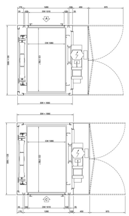
Shaft dimensions = dimensions of external structure + 50 - 0
