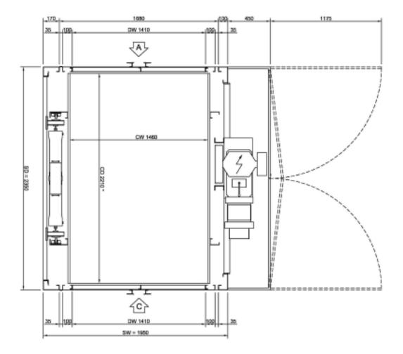
Shaft dimensions = dimensions of external structure + 50 - 0
