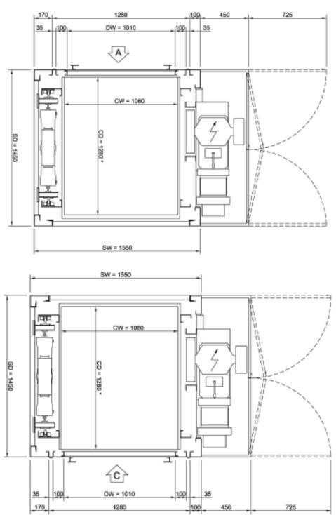
Shaft dimensions = dimensions of external structure + 50 - 0
