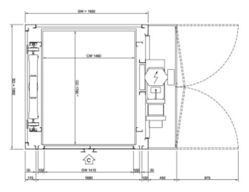
Shaft dimensions = dimensions of external structure + 50 - 0
