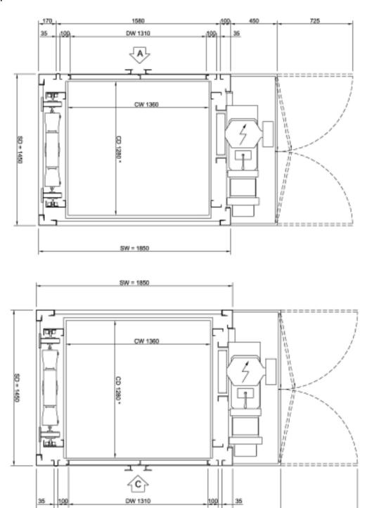
Shaft dimensions = dimensions of external structure + 50 - 0
