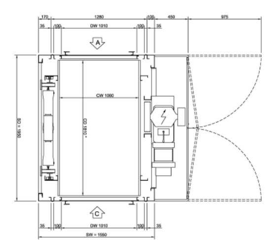
Shaft dimensions = dimensions of external structure + 50 - 0
