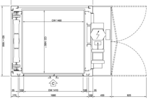
Shaft dimensions = dimensions of external structure + 50 - 0
