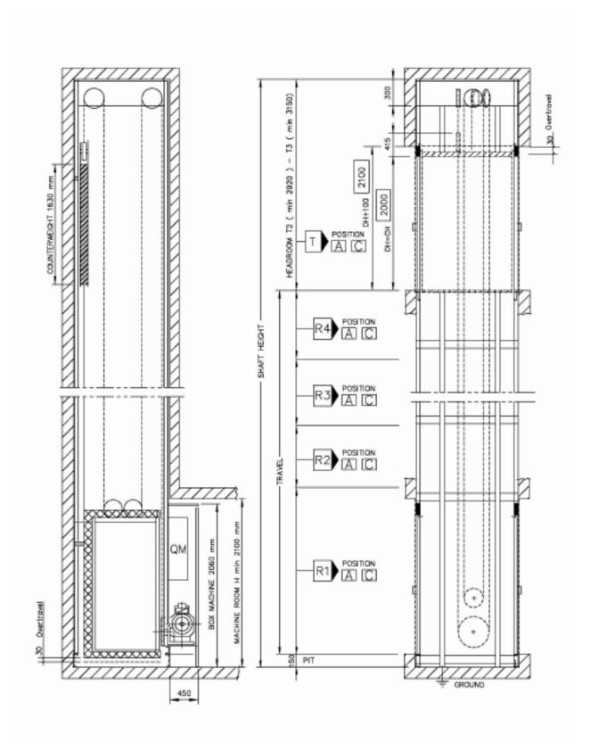
NB: Drawing only as for reference. Machine room cabinet positioned at floor different to bottom floor (OPTIONAL).
